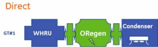
FIGURE 3 ORegen Direct Oil configuration
