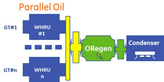
FIGURE 4 ORegen Parallel Oil configuration
