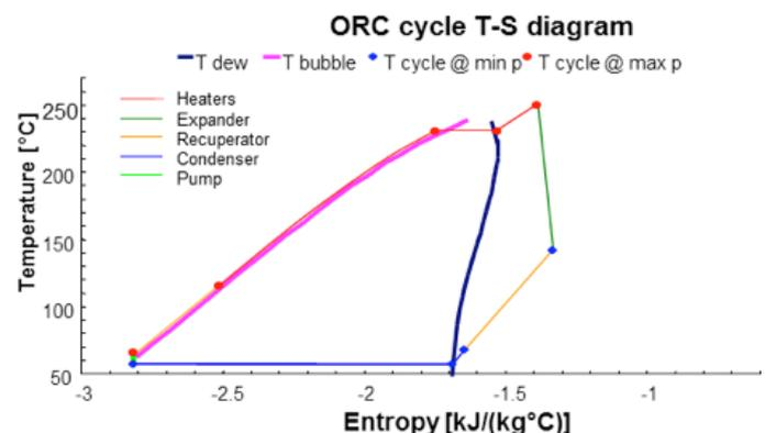
FIGURE 1 ORC T-S diagram
