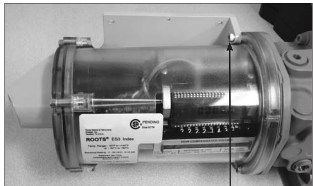
Figure 12 - Insert the 1" (long) screws 1" screws (one not shown)
