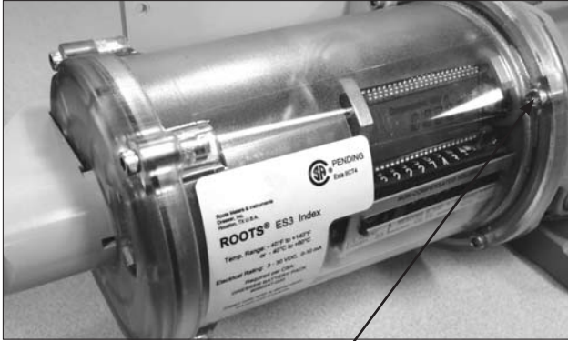
Figure 13 - Insert the 3/4" (short) screw
