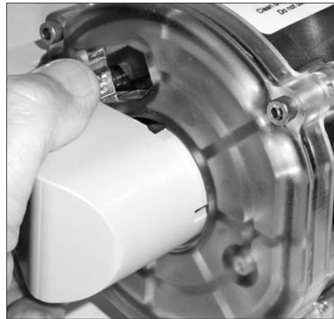
Figure 11 - Place cable gland connector into recess
