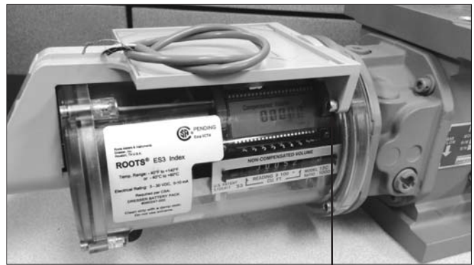
Figure 15 - insert the 1" (long) screws 1" screws (one not shown)
