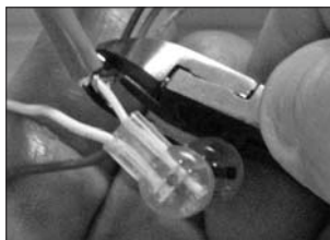
Figure 24 -Clip unused wires
