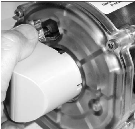
Figure 14 - Place the cable gland connector into recess
