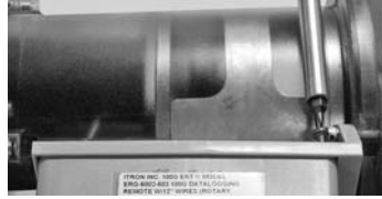
Figure 26 - Attach AMR to ES3 bracket
