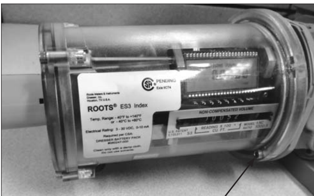
Figure 9 - Leave screw under odometer in place
