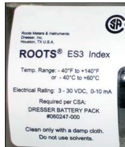
Figure 1 - Label on ES3 Electronic TC
