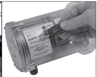
Figure 2 - Swipe magnet across the words "Roots ES3 Index" to change the screen displays
