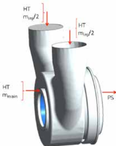
FIGURE 4 Boundary conditions scheme
