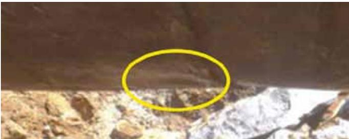
Because its slope is relatively sharp over a small area, this shallow dent has a higher strain than a deeper dent from the same inspection.
