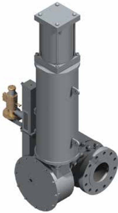
Figure 8 - Becker Surge Control Valve The Becker Surge Control Valve incorporates the Surge Design RPSR Actuator to provide protection on centrifugal natural gas pipeline compressors. The Surge Control Valve can provide stroking times less than 750 mSec.
