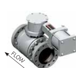
Figure 5.4 Mount #4 - Vertical Stem (Actuator Upstream) Actuator located on up-stream side of valve when looking in direction of flow (actuator horizontal/valve stem vertical).
