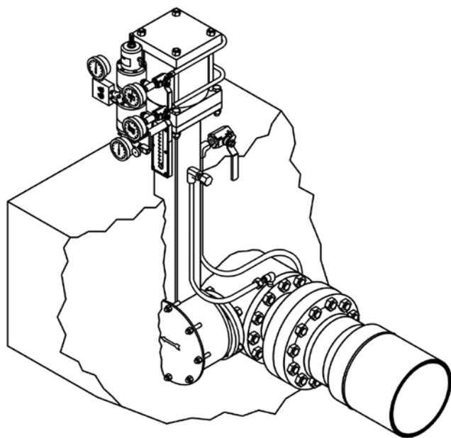
**Figure 3** - Below Ground Regulator Design Permits Easy Maintenance.
