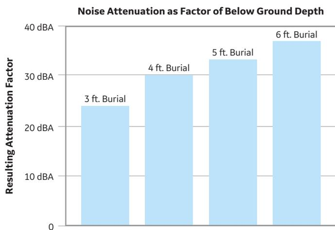
**Figure 5 -** Noise Attenuation as Factor of Depth.
