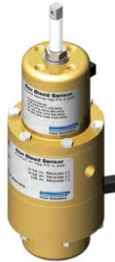
Figure 1 - Model PS-2-200 non-bleed sensor The non-bleed sensor renders Becker seat and nozzle double-acting control instrumentation non-bleeding when the corresponding control valve is at the full-open or full-closed positions. The PS-2 sensor features high pressure capabilities when power supply gas and discharge pressure gas are elevated.
