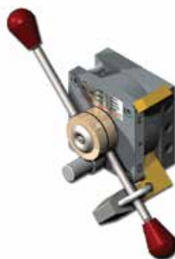
Figure 3.4 - MCV Optional Positioning Handle Locking Provision All MCV models are available with an optional positioning handle locking provision. This locking option allows the user to lock the control valve in either the full-open or full-closed position. This feature is useful during maintenance to provide lock out capabilities when it is desired to leave a valve in the full-open or full-closed position. The positioning handle locking provision may be combined with the auto/manual locking provision.
