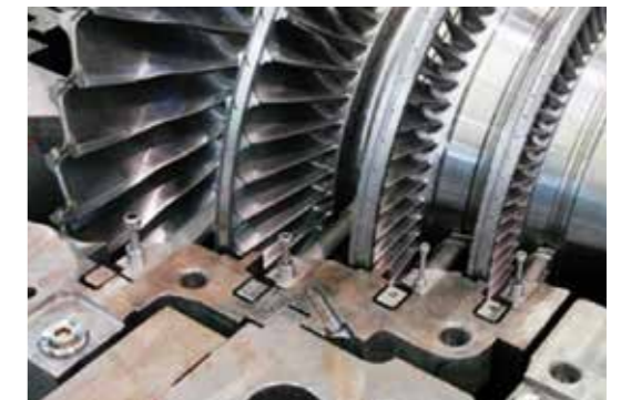
Recently developed HS low pressure stages for high speed and high efficiency applications
