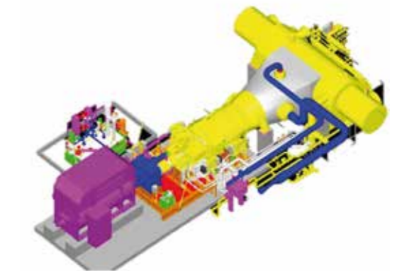
Typical STG Layout for 2xLM6000 with axial exhaust condenser... Compact layout with reduced footprint
