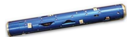
GE uses some of the highest performance IMUs available for inspection of both liquid and gas lines.
